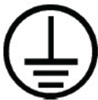
A common symbol used to identify a protective earth (PE) ground.
